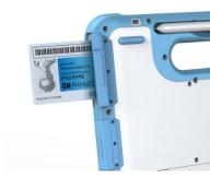
If you cannot get the CAC card reader function work properly, use different CAC card and check again. Also make sure the cards are correct type and inserted fully in the slot. If still not working, please contact your supplier for instruction
