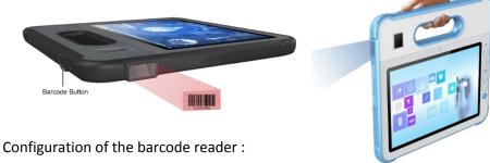
Reading the "Enter Setup" barcode may allow the engine to enter setup mode. You can then scan a number of programming barcodes to configure your engine. To exit setup mode, scan the "Exit Setup" barcode.
