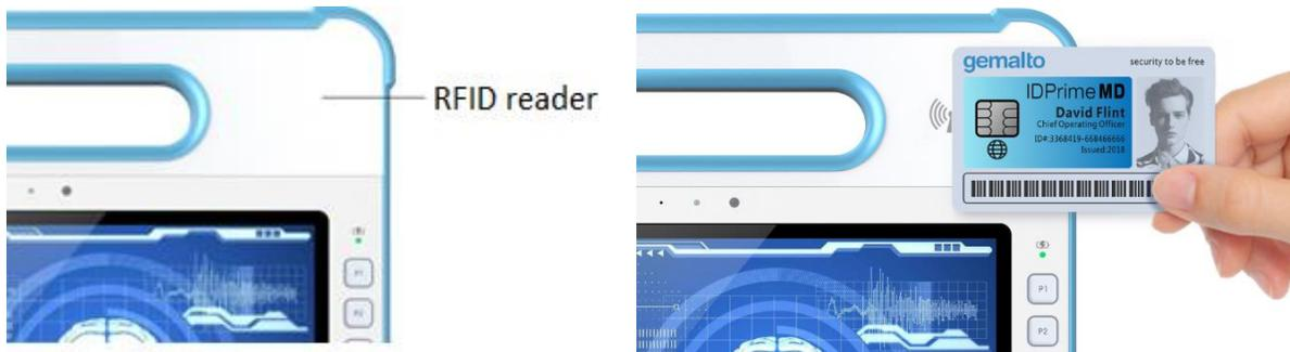
**i** The RFID tag/card must be within the range of an RFID reader. AN audible beep will indicate a successful scan.
