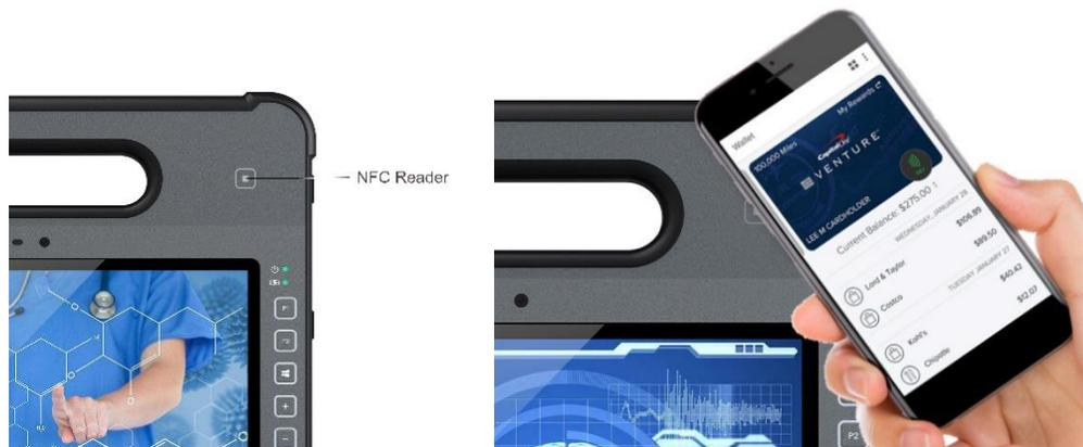
**i** Please keep the NFC tag or cards close to the NFC area within 2.5mm, otherwise the internal NFC module may not receive the signal from tag or card. If you hear a small beep, it means the scan is successful.
